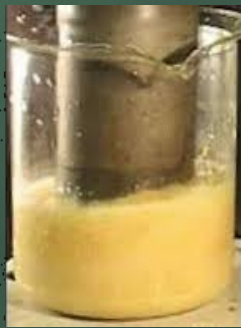
130 W, 20 kHz VCX-130 Sonics and Materials (Danbury, CT, USA) with Ti-Al-V probe (13 mm)
